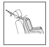
If the position you are using has an adjustable headrest or head restraint and you are using a single tether, raise the headrest or head restraint and route the tether under the headrest or head restraint and in between the headrest or head restraint posts.
